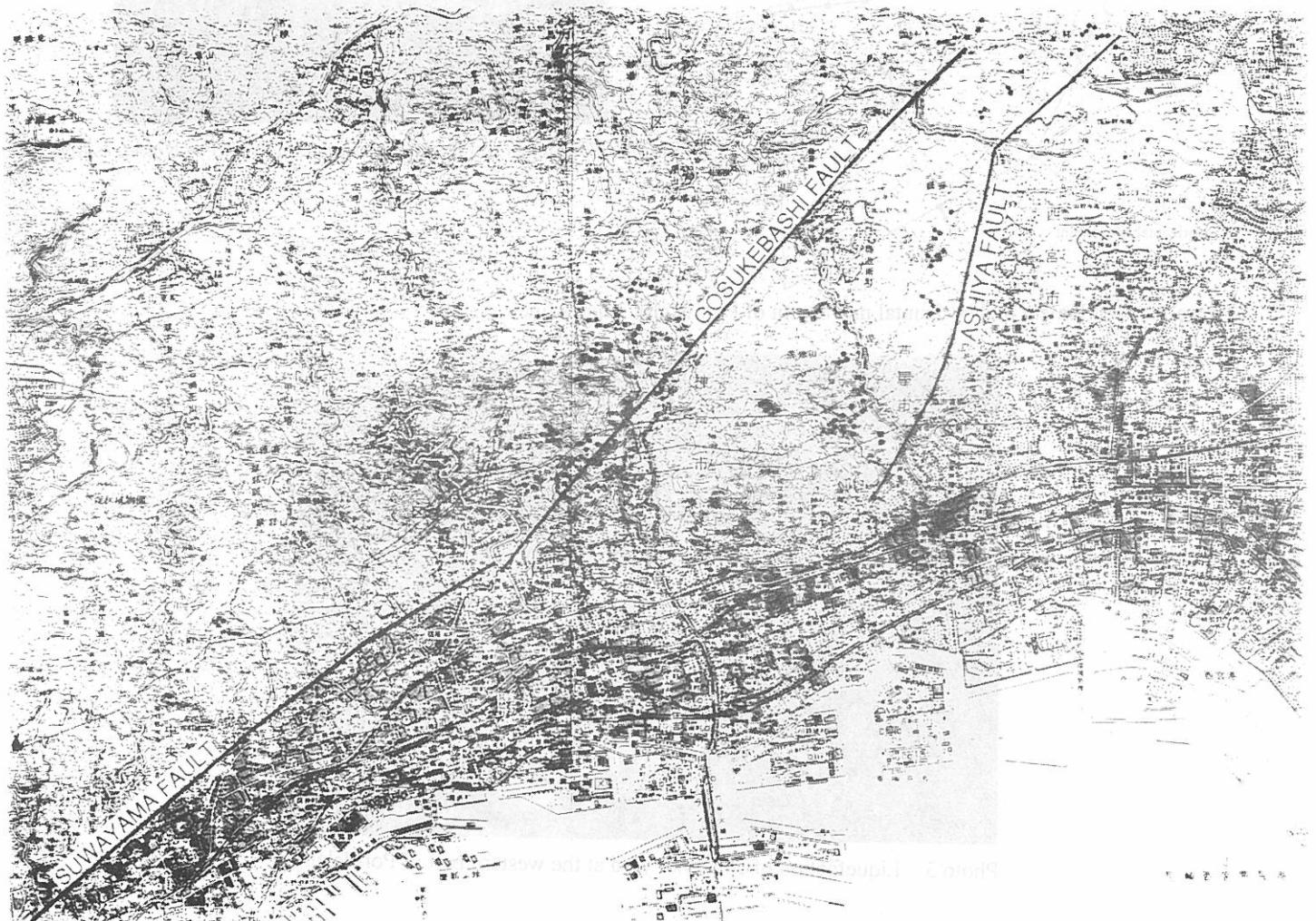
Figure 13 Distribution of the mountain slope failures at the eastern part of the Rokko mountains
