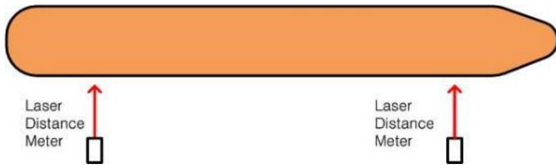
Fig. 2.2 Arrangement of Dock Mounted Laser System
