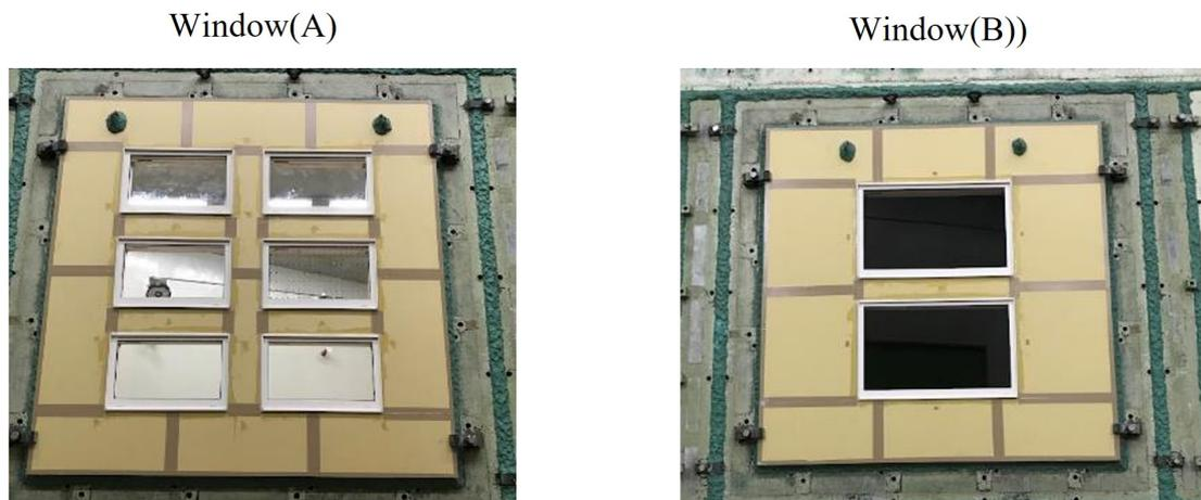
Figure 5.3: Multiple windows attached to wooden frame. **(left)**: Attach six windows to wooden frame in measuring case of window(A). **(right)**: Attach two windows to wooden frame in measuring case of window(B).
