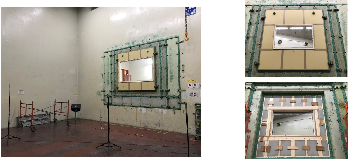
Figure 5.1: The picture of sound insulation test. (left) : Measurement occasion in laboratory seen from sound reverberant room. (upper-right) : Measured sample window (C) seen from sound room. (bottom-right) : Measured sample window (C) seen from receiving room.
