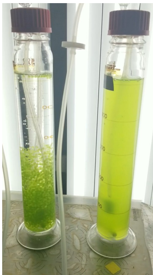
Figure 2. Experimental setup for the culture of immobilized cells (left flask) and free cells (right flask) of Chlorella sorokiniana .
