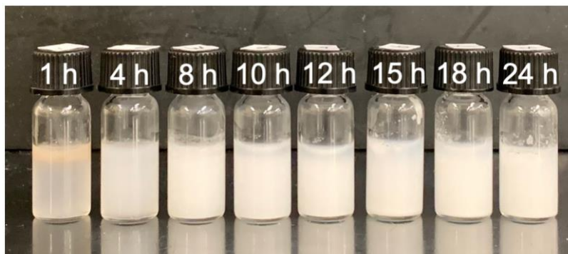
Figure 9. Evolution appearance of PVAc dispersions prepared by ms ITP using V-70 as initiator at 30°C.
