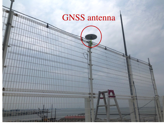
Figure 4.1: Data collection by a fixed GNSS antenna. The antenna is located at 34.7136832 [deg] north latitude and 135.3353441 [deg] east longitude. There are few obstacles around the antenna that block direct signals from satellites.
