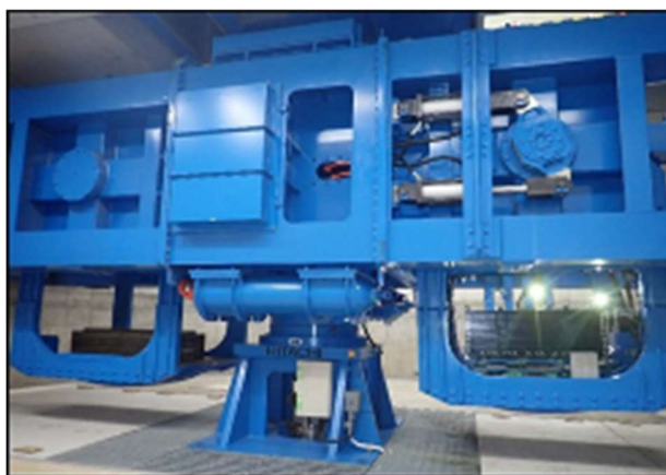
Fig. 3-1 Geotechnical beam centrifuge at the National Agricultural and Food Research Organization in Japan
