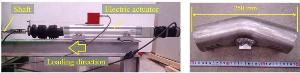
(a) Loading equipment
