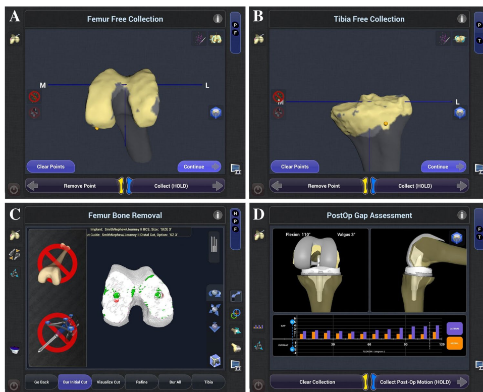
Fig. 2 Feature of handheld robot. A Bone surface registration. Bone surface of the femur was morphologically registered by morphing and painting technique with the probe. B Surface registration of the tibia by morphing technique. Bone surface of the tibia was also morphologically registered by morphing and painting technique with the probe. C Distal and anteroposterior femoral cut. Distal femoral shaving was performed, in which targeted cut surface was changed from purple, green, to white color, with a high-speed 5-mm burr. This burr
