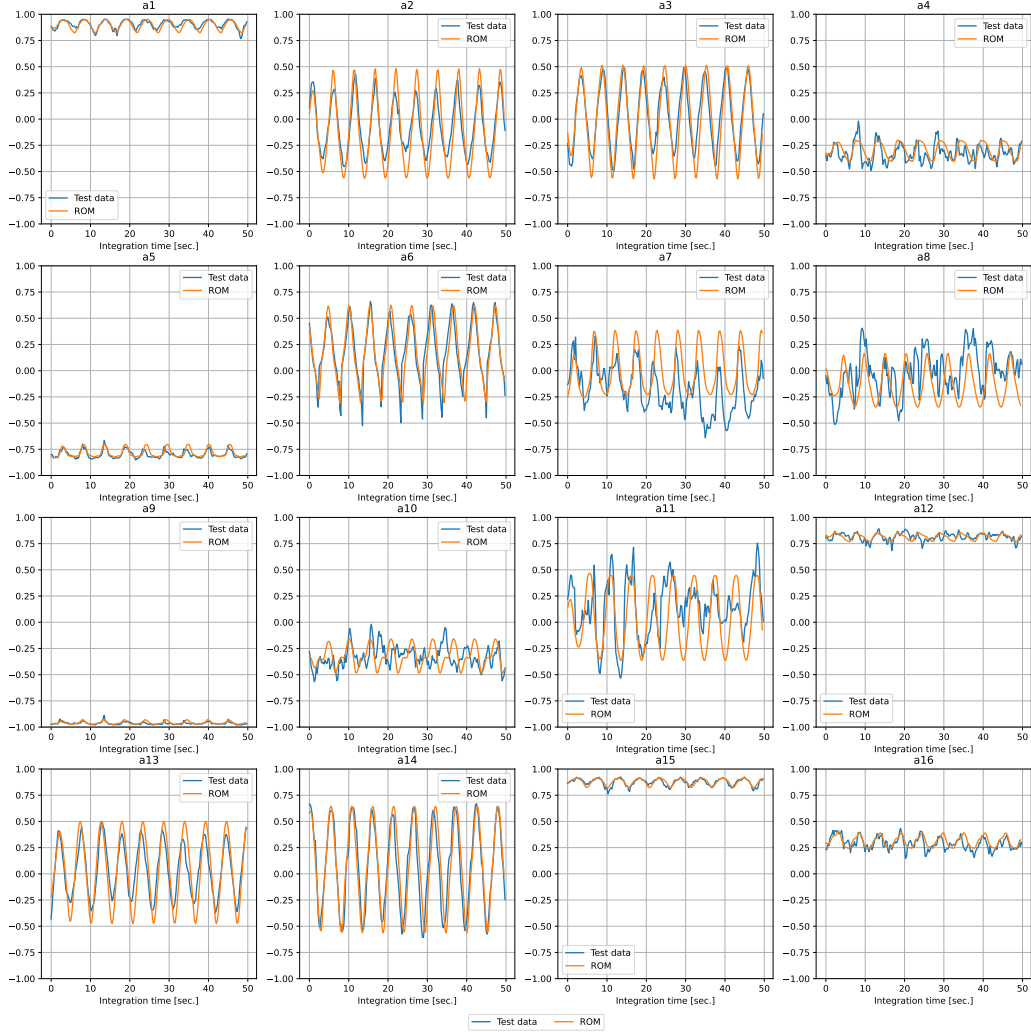
Figure C.27: Time series of latent vector elements predicted by LSTM with 16 modes-decomposition: the blue and orange lines indicate the test data and the prediction with LSTM derived from first 20 time steps.
