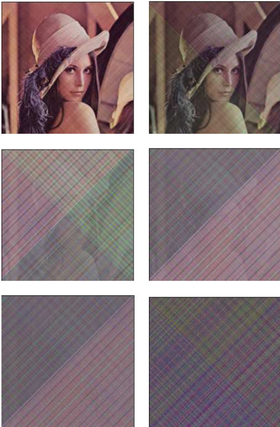
Fig.2.20 The effect of changing the m value in the modulation and demodulation portions on the image encryption effect. Six different values of m ( m = 1.0, 2.0, 5.0, 6.0, 7.5, 8.8 ) were tried, and the corresponding encryption effects were observed for each, where the larger the value of m , the better the secrecy performance of the image, within the computable range.
