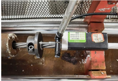
Fig. 2.21 Steel plate and displacement transducer
