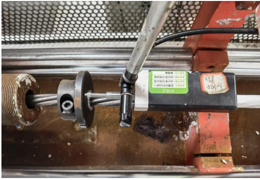
Fig. 2.4 Steel plate and displacement sensor
