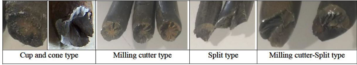
Fig. 2.27 Fracture type of corroded steel wires [47]
