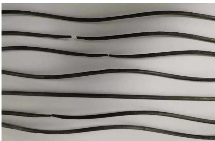
Fig. 2.7 Disassembled corroded steel wires
