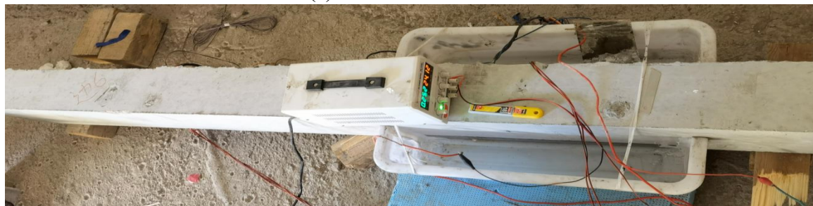
(b) Corrode at side
