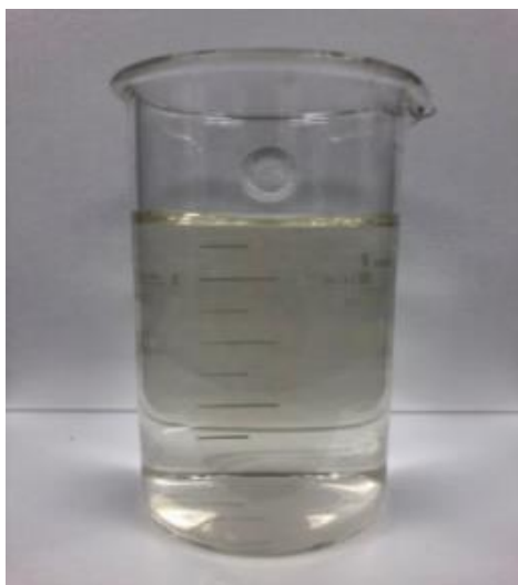
Fig. 4-8 Electrochemically oxidized liquid digestate with a Pt-Co value of 200
