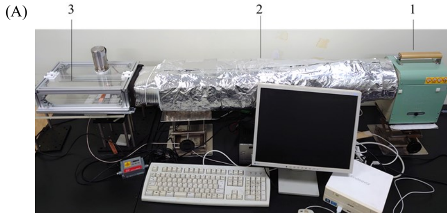
1. Hot air generator, 2. Insulated duct, 3. Drying chamber
