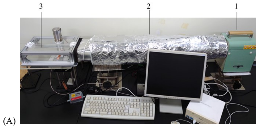
1. Hot air generator, 2. Insulated duct, 3. Drying chamber
