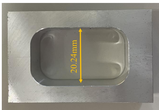
Fig. 22 Through pocket machined without modification and width of center of the pocket.
