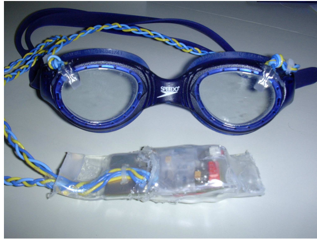
Fig. 1. Goggles with one bi-color LED[2]
