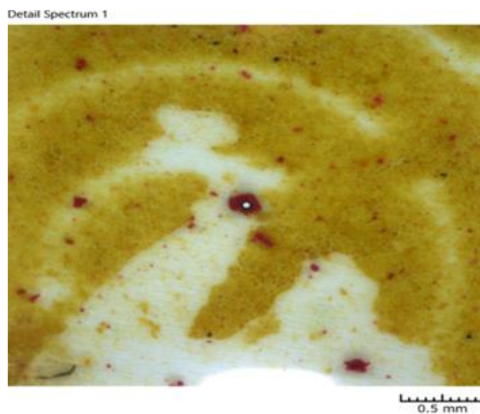
Fig.5-1 The abundance of Cu-Zn-based APPs (>150 \mu\text{m} ) fell from painted-steel samples
