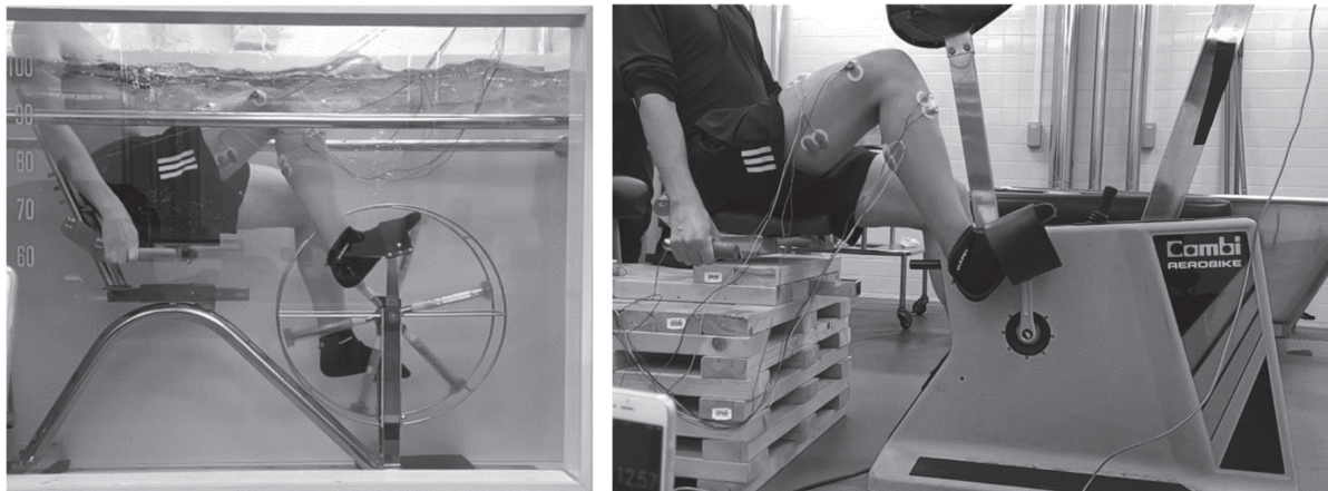
Figure 2. Muscle Activity Measurement: The saddle position of the recumbent ergometer was adjusted. Participants were instructed to keep their backs off the backrest and hold onto the handlebars on either side of the saddle. Additionally, the right pedals were adjusted such that the right knee joint flexion was 90° at the uppermost point (0°). After pedalling exercise was stabilized, EMG data were recorded for 10 rotations during the pedalling exercise.
