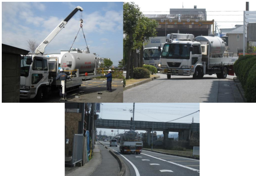
Fig.3 Photograph of transportation test of 2000 liter LH 2 tank by truck.
