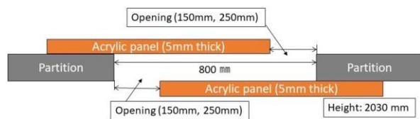
Figure 2: Sketch of the cross-sectional view of the mockup plenum structure used in the experiments.
