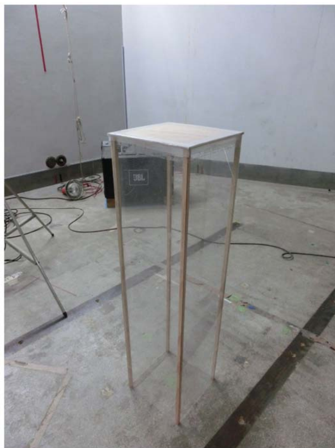
Figure 1. A photograph of the specimen of RMSA used in the experiment (number 1 with a removable cover on the top end)
