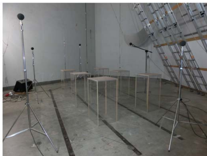
Figure 2. The specimens of rectangular MPP space sound absorbers (RMSA) set in a reverberation chamber. In this photo the top ends of the specimens are closed with removable covers
