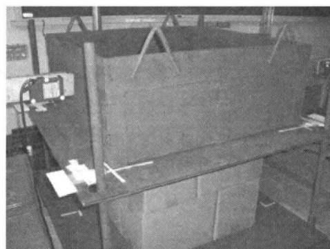
Fig.8 Stacking Test on 4c/s Pin-wheel Tier(2stairs)
