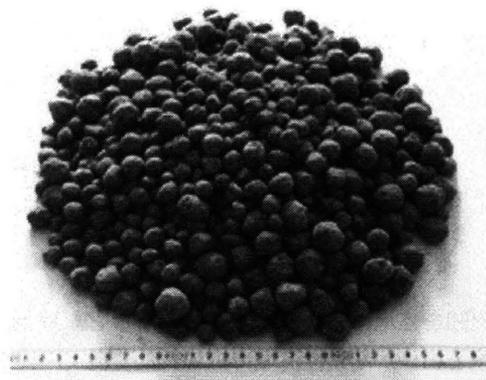
Fig.1 Photograph of Granulated Coal Ash (GCA)
