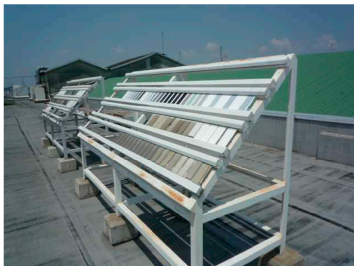
Figure 3. Outdoor exposure test at Osaka.
