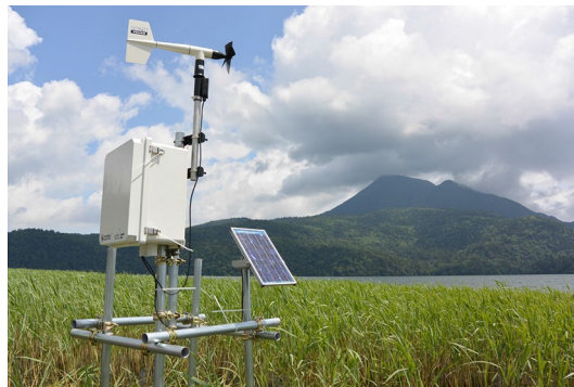
Figure 10. Meteorological station for measuring wind speed and direction at Churui Bay in Lake Akan.
