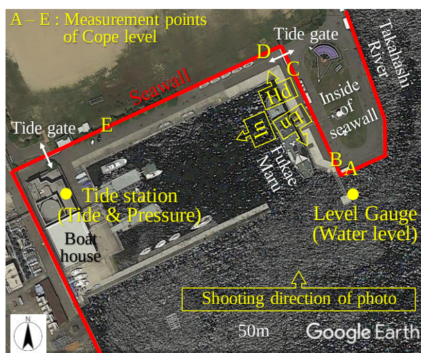
(c) Seawall, survey points and so on around Fukae harbor. In means the inner part of the harbor, Hd means heading ward of Fukae Maru and En means entrance ward of harbor in shooting direction of photo shown in Fig.3.
