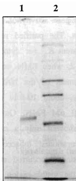
Fig. 2-1. SDS-PAGE analysis of the purified tobacco NADPH-cytochrome P450 oxidoreductase. Polyacrylamide gel concentration was 7.5%. Lane 1: NADPH-cytochrome P450 oxidoreductase after chromatography on a DEAE-Toyopearl column (0.5 \mu\text{g} ). Lane 2: standard molecular weight marker (2.0 \mu\text{g} ): myosin ( M_r 205,000); \beta -galactosidase ( M_r 116,000); phosphorylase b ( M_r 97,400); albumin, bovine ( M_r 66,000); albumin, egg ( M_r 45,000).
