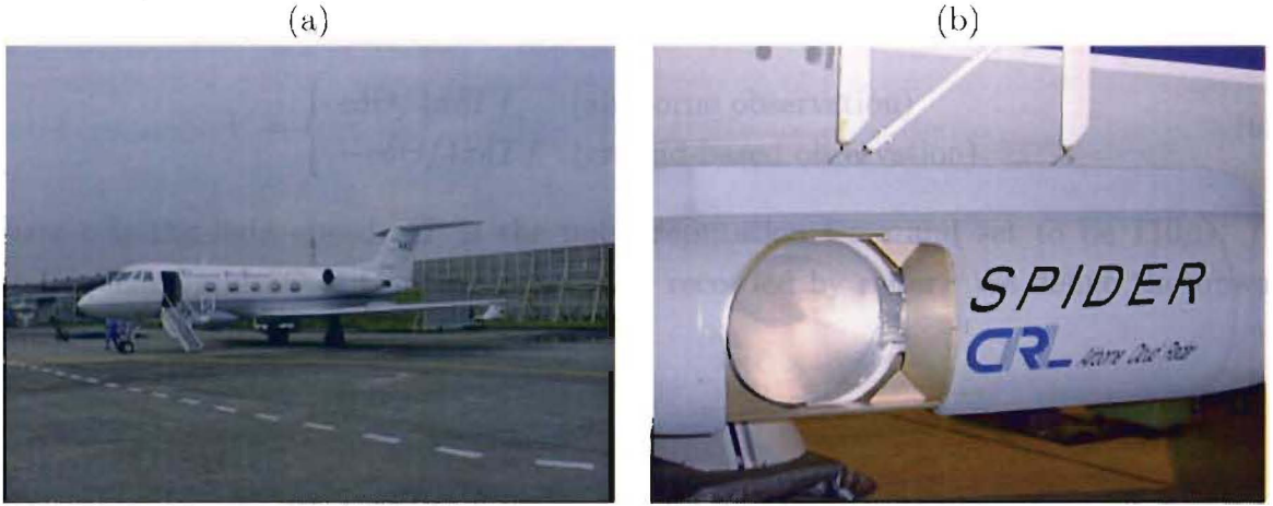
Figure 6.1: (a) SPIDER installed in an aircraft, Gulfstream II. (b) magnification of radar in (a).
