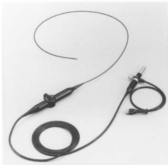
FIG. 1. The AF-22 had an external diameter of 2.2mm, an effective length of 1000mm, a visual angle of 75°, and an observation depth of 2 to 50mm. The tip of the AF-22 could be bent 120° both upward and downward and had one channel.
