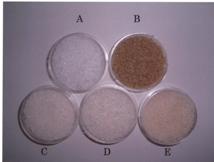
Figure 3-6. Photograph of obtained sugar A: Granulated sugar, B: Raw sugar (made in Australia), C: A-sugar, D: B-sugar, E: C-sugar
