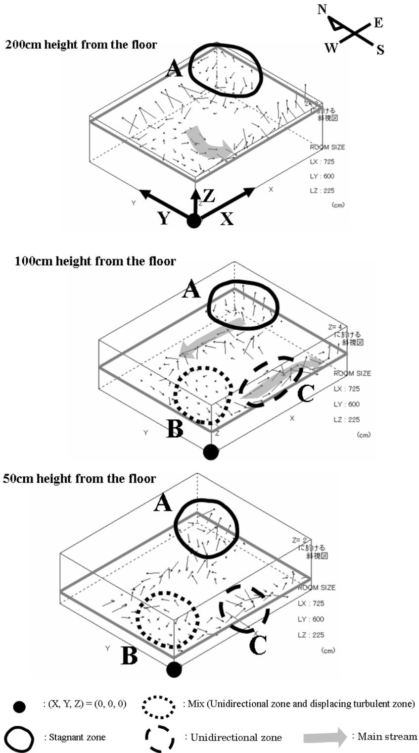
Figure 2-5. The second measurement of three dimensional air velocities
