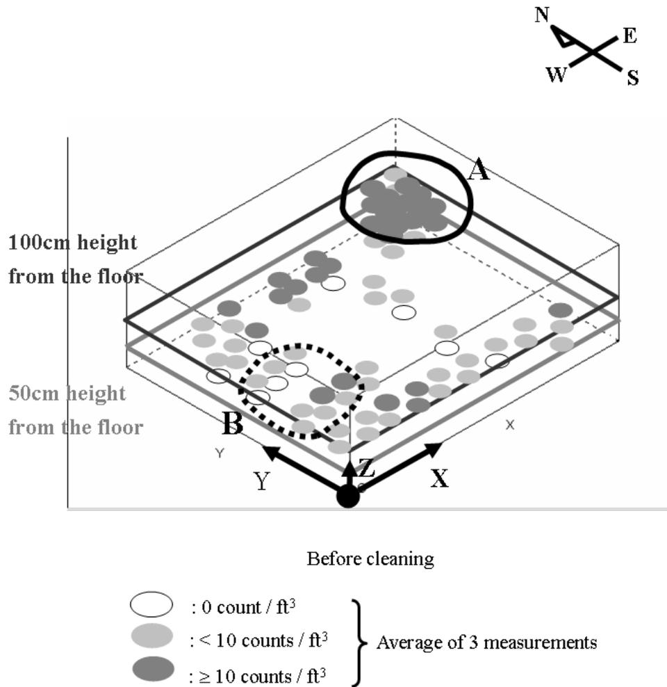
**Figure 2-7. The distributed particle concentrations before cleaning**
