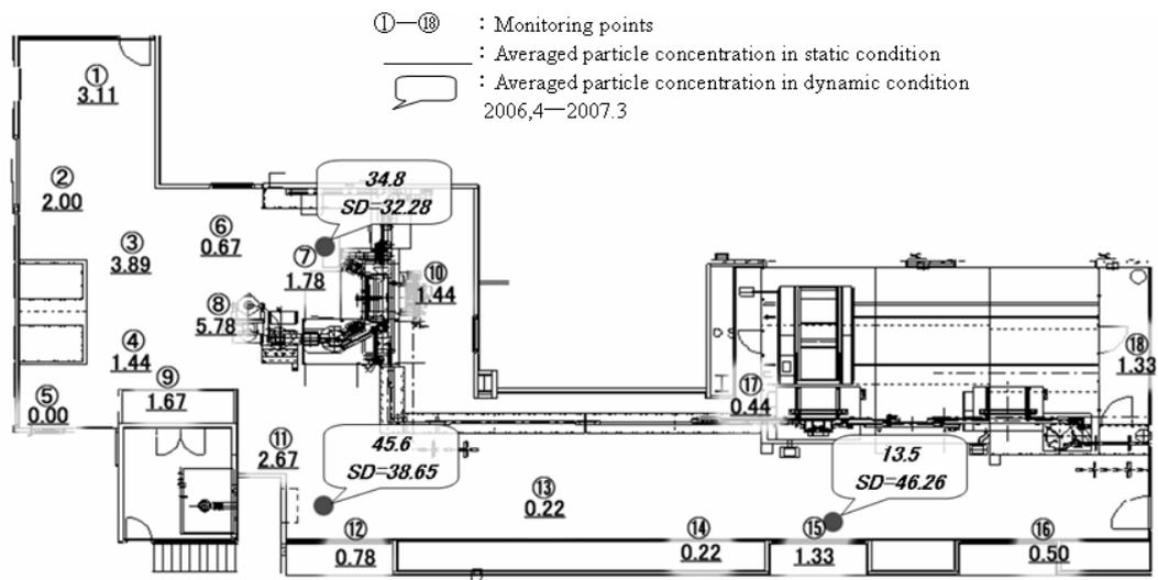
**Figure. 4-1 Air born particle concentration at each monitoring points in aseptic manufacturing room (0.5 $\mu$ m)**
