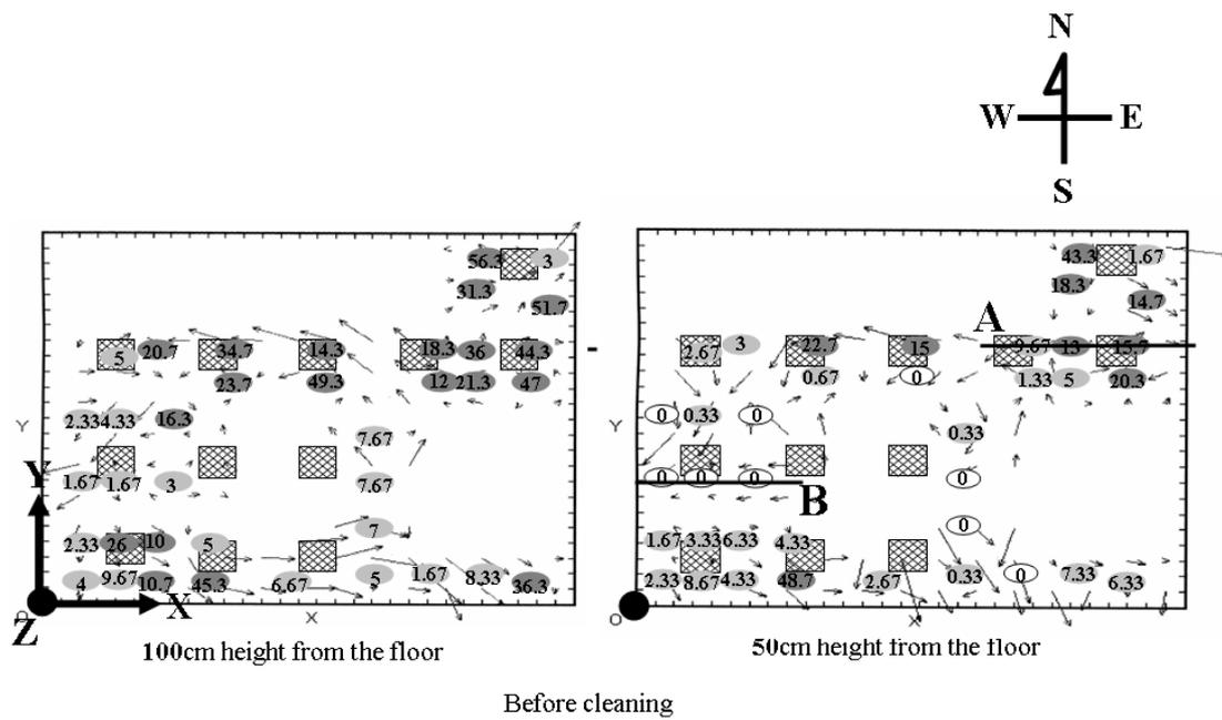
**Figure 2-6. Airborne particle counts before cleaning**
