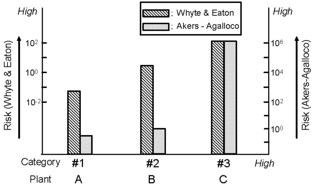
**Figure 5-1. Risk score comparison used two risk assessment tools in three existing facilities. A significant gap is observed between Plant C and Plants A, B**
