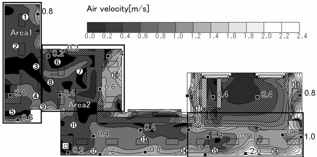
**Figure. 4-2 Simulated distribution of air velocity**
