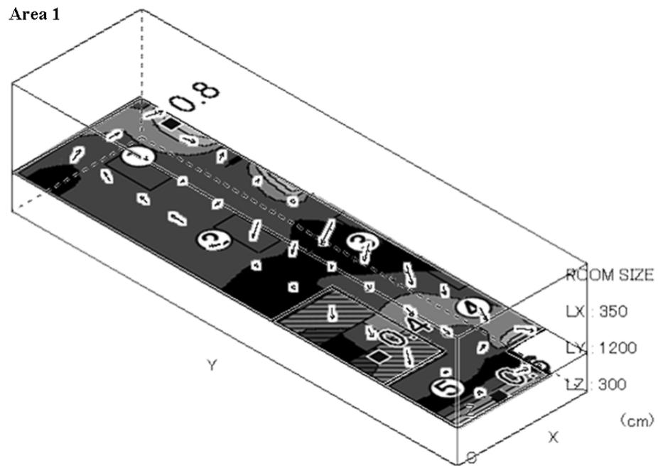
**Figure. 4-3 Actual air vectors and simulated distribution of air velocity in**
