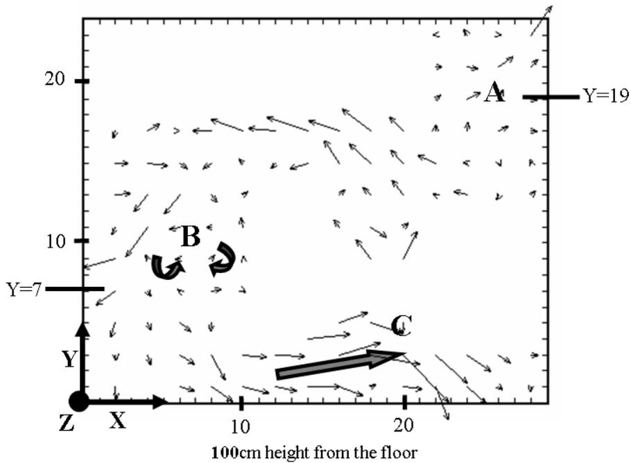
**Figure 2-8-2. Airflow pattern of the top view at 100cm height from the floor**
