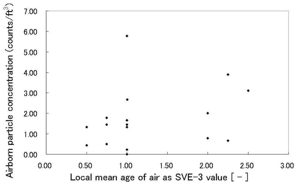
Figure. 4-8 Relationship between local age of air as SVE-3 value and particle concentration at each monitoring points
