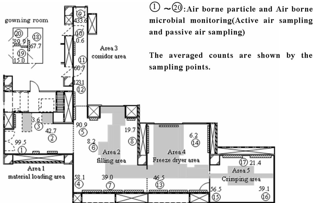
Figure 3-2. Average of 0.5µm airborne particle counts at the height of 50, 100 and 200 cm for 9 days
