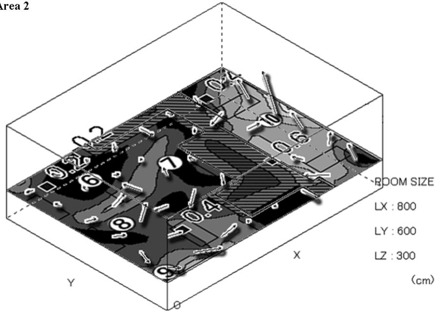
Figure. 4-4 Actual air vectors and simulated distribution of air velocity in
