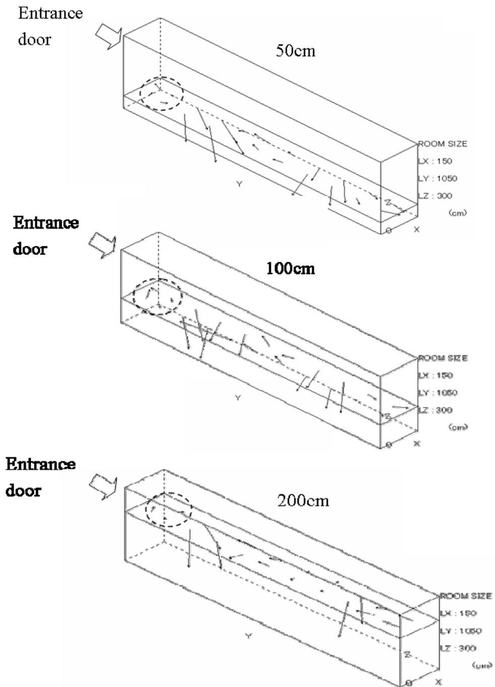
**Figure 3-3-2. Airflow vector diagram of the Area 3 Filling area at 50, 100 and 200 cm above ground**
