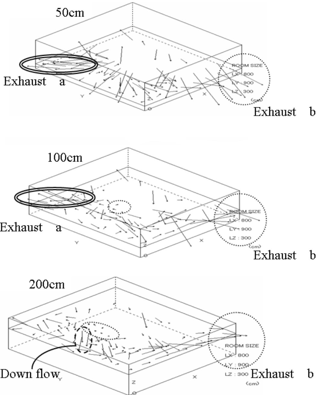
**Figure 3-3-1. Airflow vector diagram of the Area 2 Filling area at 50, 100 and 200 cm above ground**
