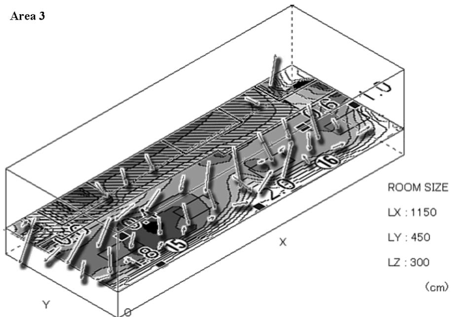
Figure. 4-5 Actual air vectors and simulated distribution of air velocity in
