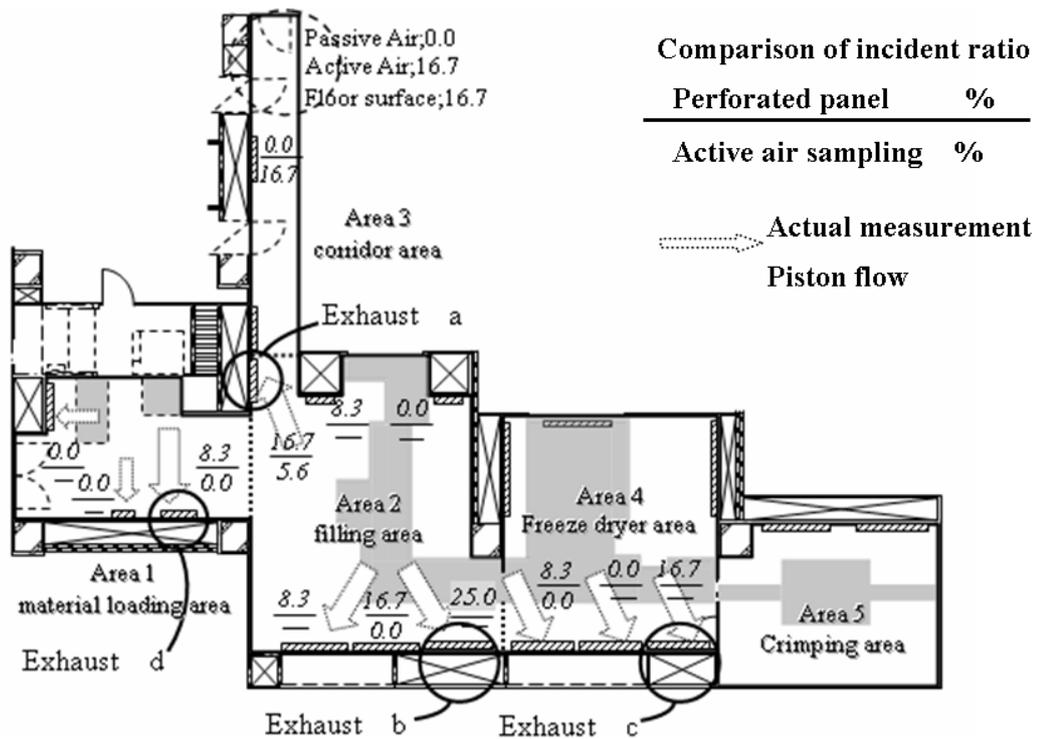
**Figure 3-5. Comparison of the incident ratios from air sampling and surface sampling during Days 4-9**
