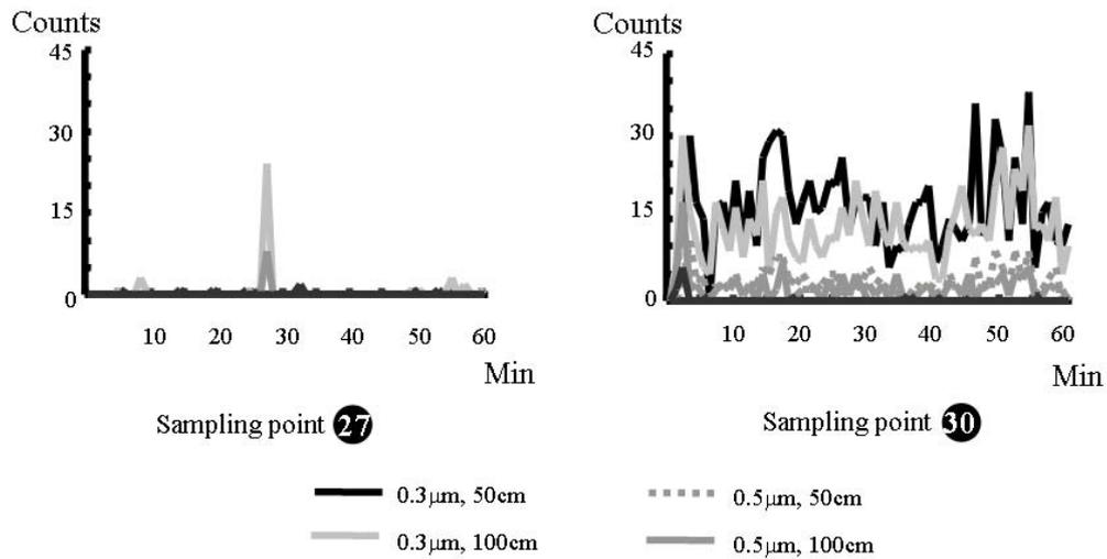
**Figure 2-12. Airborne particle continuous monitoring**
