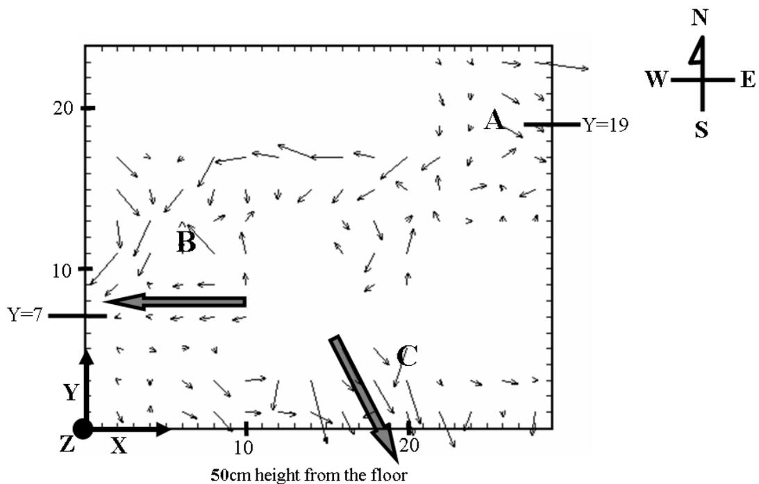
**Figure 2-8-1. Airflow pattern of the top view at 50cm height from the floor**
