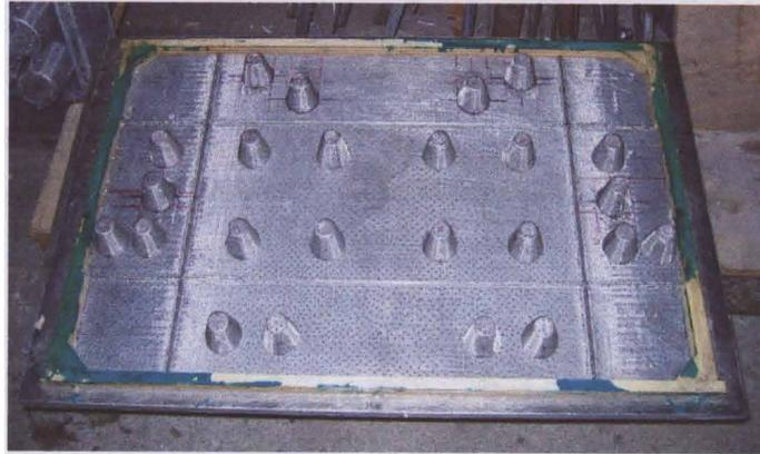
**Fig.5.13 A sample of the mold tool for a gas appliance**
