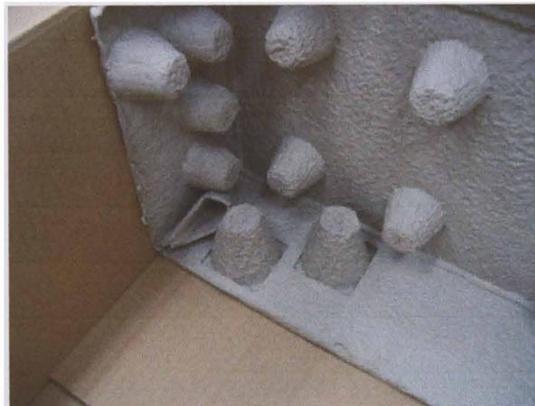
**Fig.5.20 A condition of the cushioning after the transport test**
