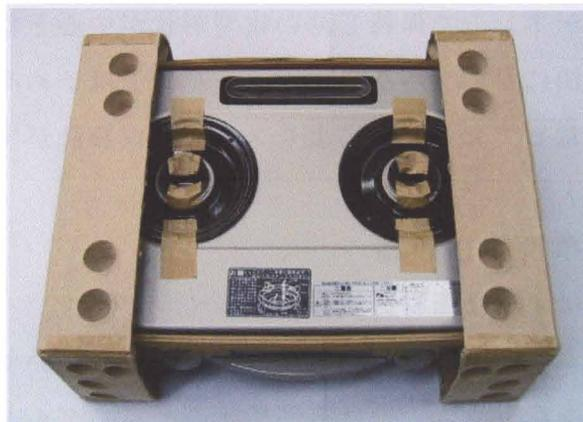
**Fig.5.15 A gas appliance set up on the cushioning**
