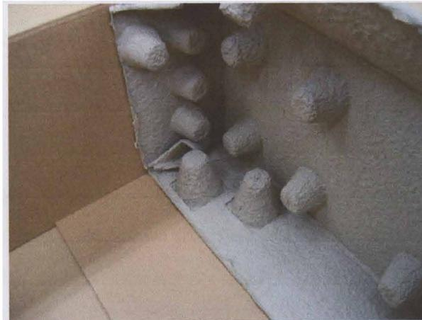
**Fig.5.19 A condition of the cushioning before the transport test**
