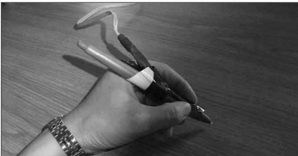
Fig. 1. Grip force measuring writing device
