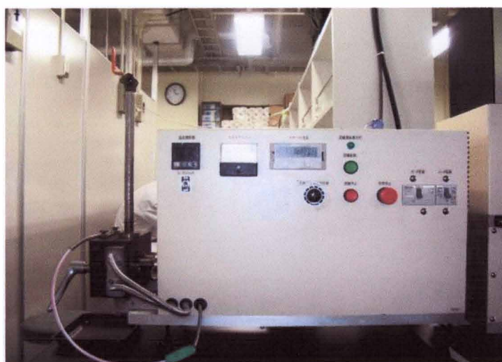
Fig. II.3. Mixer with a twin blade for cloud point sample.
