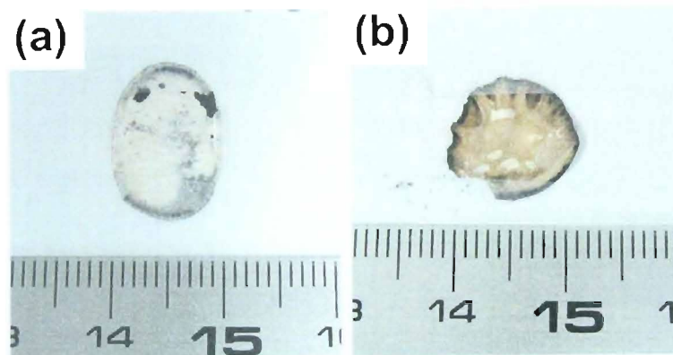
Figure 2.1.13 Photographs of the (a) Celgard membrane and the (b) PAN nonwoven after the hot oven test at 150 °C.
