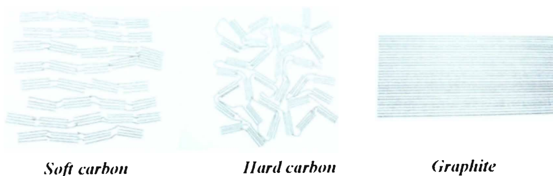
Figure 1.8 Three types of carbon used in lithium ion battery.
