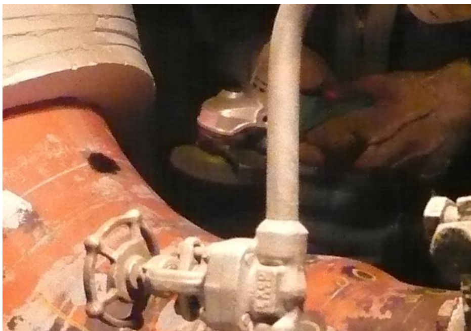
Fig. 1.2.1-5: Preprocessing for UT. The coating needs to be removed, because pipe coating thickness affects the thickness measurement.
