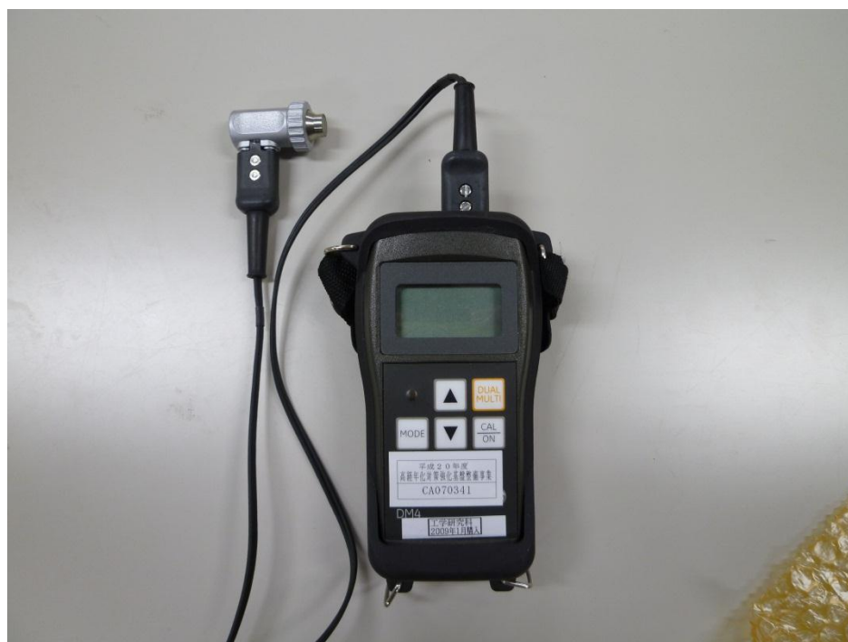
Fig. 2.2.1-2: Wall thickness gage using PZT
