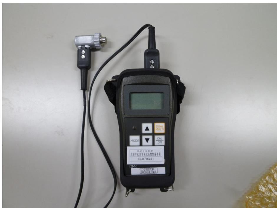
Fig. 2.2.1-2: Wall thickness gage using PZT
