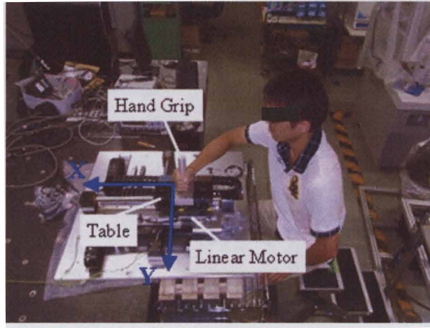
Fig. 5.6 Measuring equipment of iteration numbers for keeping constant force with interval
