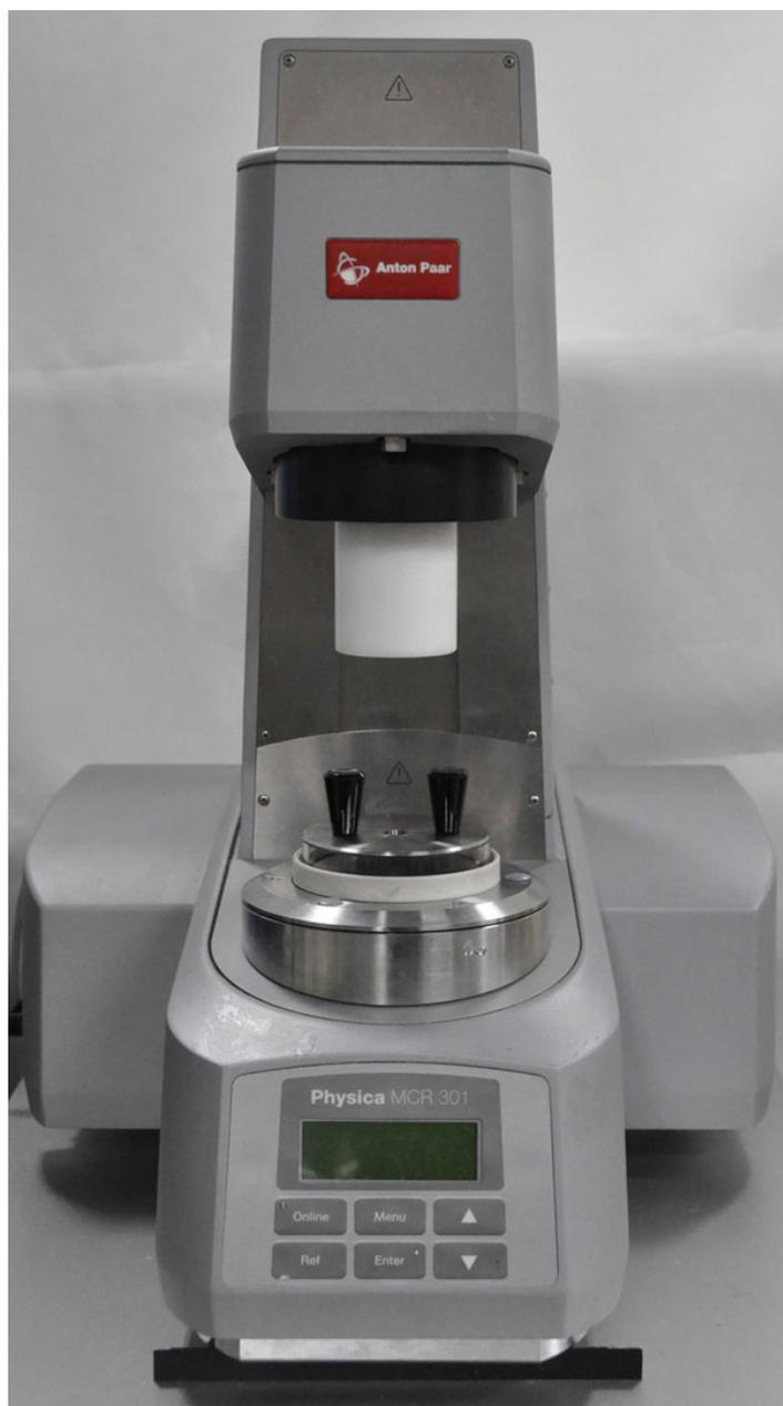
Figure 3.6 Stress controlled Rheometer MCR-301 (Anton Paar).
