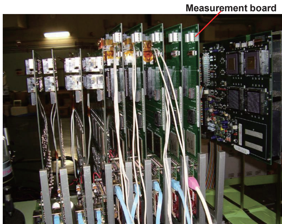
Fig. 5.12 Photograph of neutron accelerated test.
