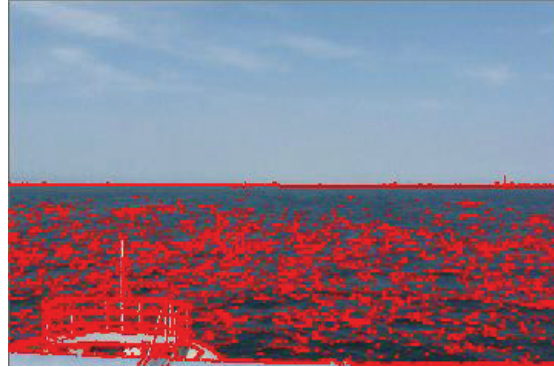
Fig.7-8 Sobel edge detection with horizontal, vertical and diagonal components
