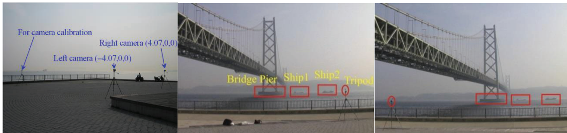
Fig.3-1 Experimental stereo configuration and obtained left and right images
