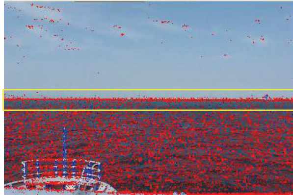
Fig.7-6 Result of Sobel edge detection on non-filtered image
