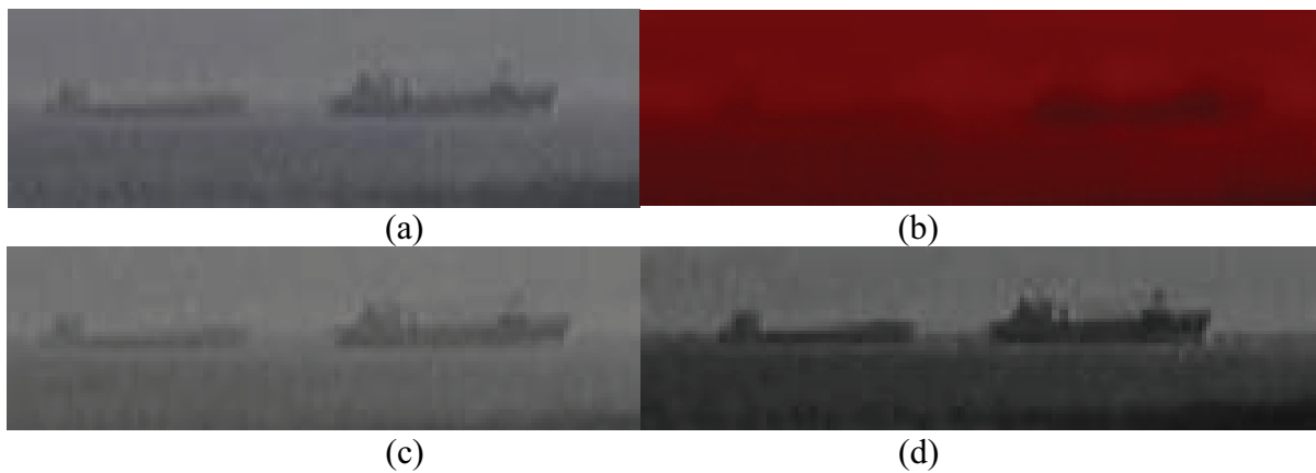
Fig.8-2 Magnified ship images (a) Original (b) Red channel only (c) Gray level (d) Histogram Equalized gray level
