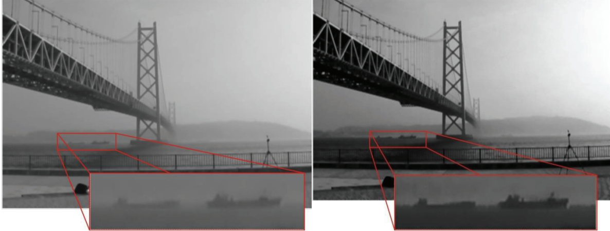
Fig.8-4 Application of bilateral filter to gray scale and histogram equalized image
