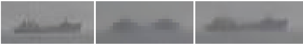
Fig.5-6 Effect of filtering on ship image a) Original b) Median filtered c) Bilateral filtered
