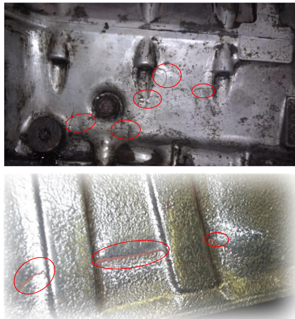
Figure 4.1 Surface cracks of engine block
