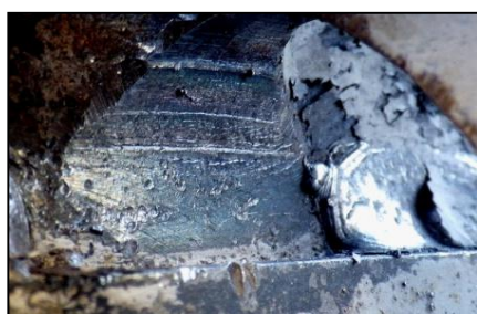
(a) BS-29: Crack initiation(at +3.0 \theta_p )
