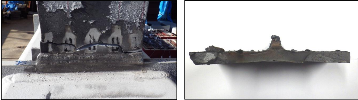
Fig. 2.14 Typical final failure mode
