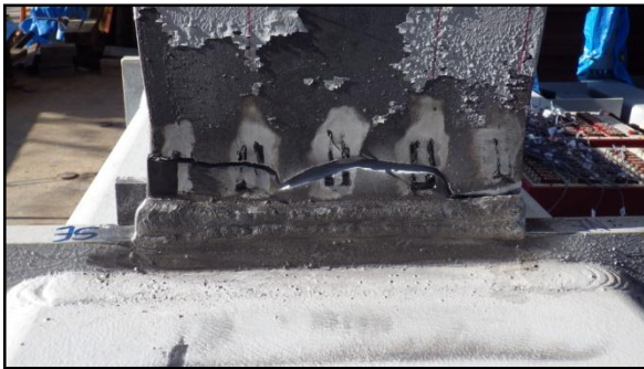
(a) Ductile fracture
