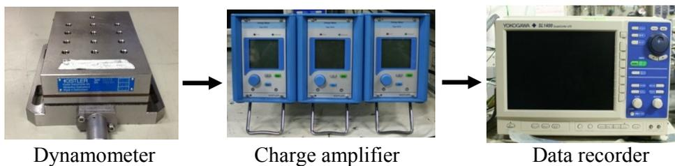
Fig.5.2 Experimental equipment for cutting power measurement
