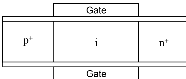
Fig. 6.1 Device structure of TFET. Unlike conventional MOSFETs, acceptors are injected to the source for n-type TFET.
