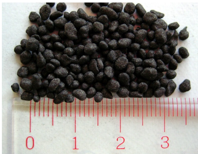
Figure 1: Photograph of the granulated Ni(OH) 2 particles.
