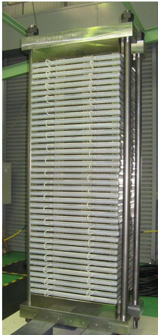
Figure 10 the extremely large-sized battery stack with 40 cells and 1500Ah (75kWh).
