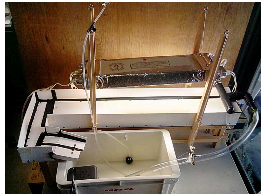
(b) Picture of the PBR after the construction. The project have been slightly varied to comply with the laboratory layout.
