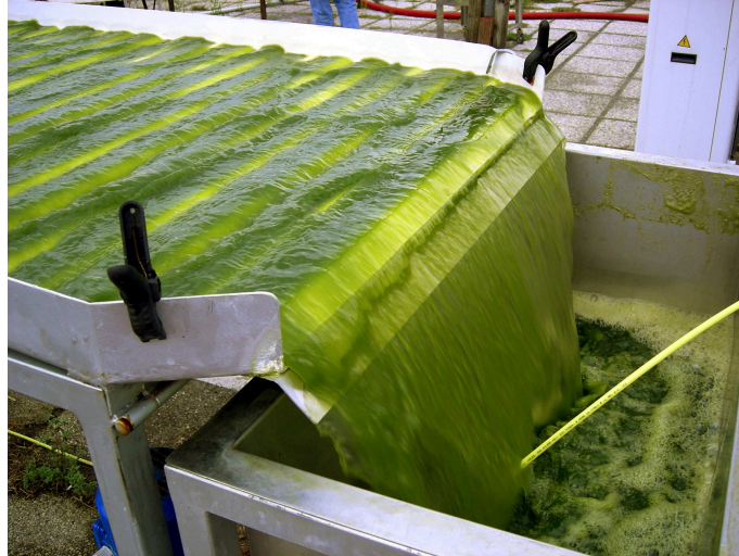
Figure 6.6.1: Chlorella s. growing in the outdoor cascade photobioreactor in the ISE facility (Florence)
