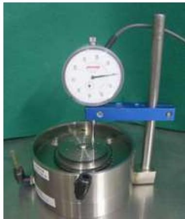
Photo A-1 Measuring instrument of resin expansion
