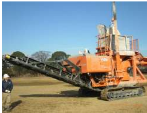
Photo 3.1 SR-G2000 Track Mounted Soil Recycler
