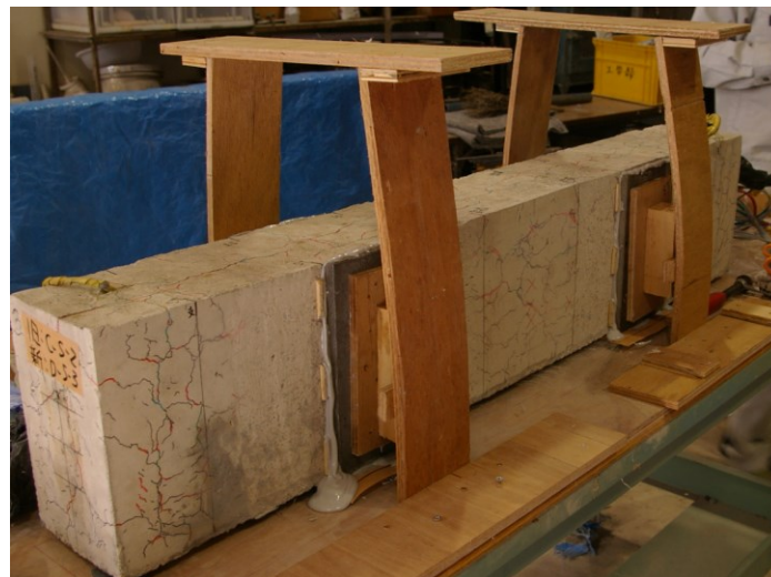
Fig. 5.20. The photo of UFC panel bonding.
