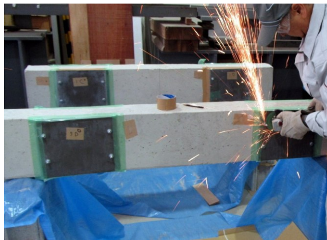
Fig. 4.4. Setting of UFC panel.
