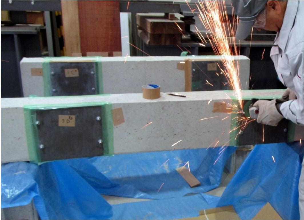
Fig. 2.4. Setting of UFC panel.
