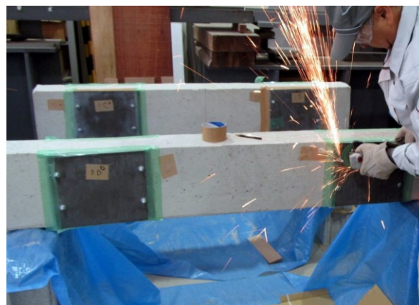
Fig. 3.2. Setting of UFC panel.
