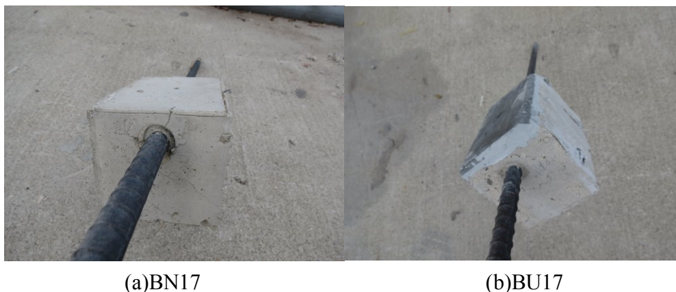
Fig. 3.15. Photos after bond-slip tests.
