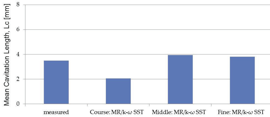
Figure 8.4: Measured and calculated mean cavitation lengths with different mesh sizes at P_{inj} = 0.22 MPa
