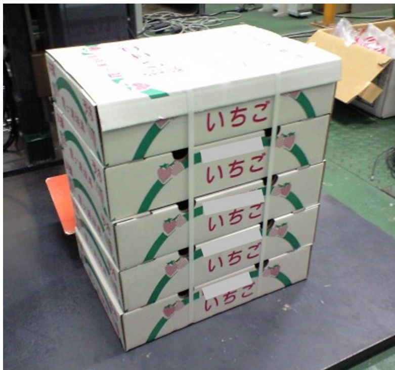
Fig. 5-2 Form of packaging for estimation of PAcc , Vc , and fruit damage
