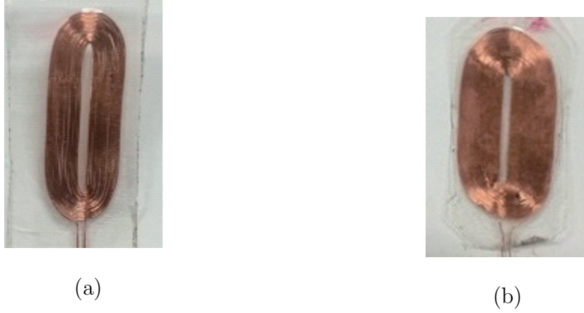
Fig. 4.3: Coils for the EMAT used in the guided wave testing system. (a) is for transmitting EMAT ring array, (b) is for receiving EMAT ring array.
